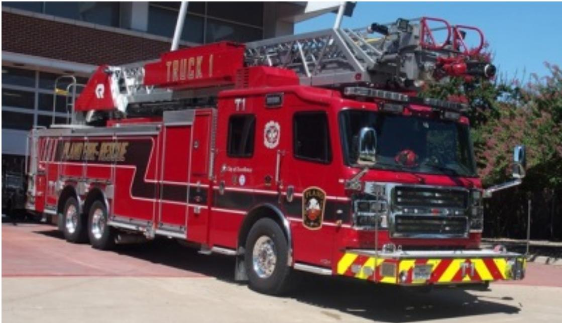
Truck 1 - 2014 Rosenbauer / Waterus 1250 GPM Pump, 300 Gallon Tank, 109 Foot Aerial Ladder
