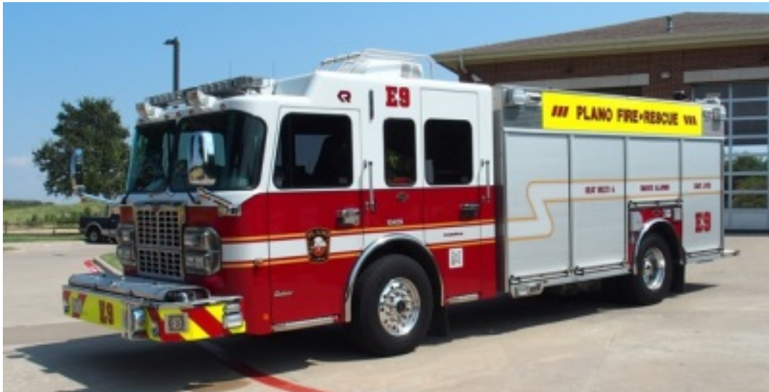
Engine 9 – 2008 Spartan / Rosenbauer 1250 GPM Pump, 500 Gallon Tank, CAFS
